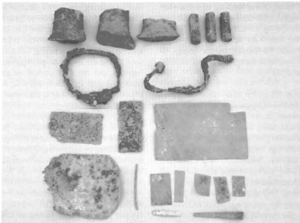
Photo 31. Raw materials recovered from the New York Knife Company factory. Top row is pig iron and steel rods. Second row is square spring steel wire. Bottom row is pieces of sheet steel and brass. The three steel rods in the upper right of the photo are 5 cm (2 in.) in length.
