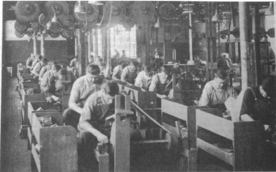
Historic Photo 4. Early twentieth century photo of a grinding room in a knife factory. (Voyles 1995 by permission of Krause Publication)
