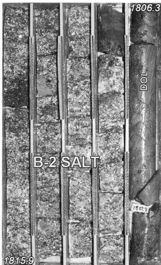
Photograph 1: Rotated blocks of dolostone and shale at top of B2 salt bed in core from Hampton Corners hole 9456 (API #21576). Note near-vertical laminae within dolostone interval below 1,806.6 feet.
