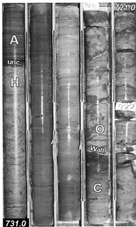
Photograph 7: Bertie Group transition from the wispy-mottled top of Unit H ( H ), through Akron ( A ) and Cobleskill ( C ) Formations, and into the cherty Edgecliff Member of the Onondaga Formation ( O ), above the Wallbridge Unconformity ( Wall. ). Core is from Hampton Corners hole 9443 (API #21557).
