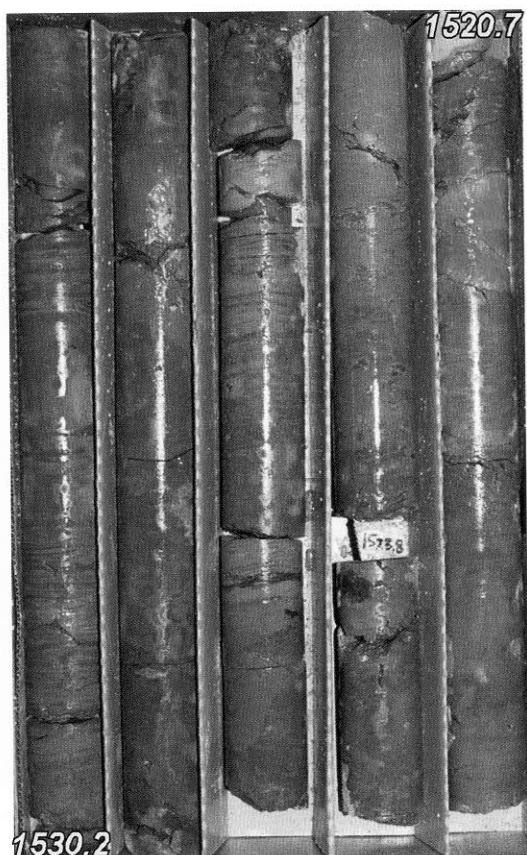
Photograph 3: Red and green shale of the Vernon Unit C formation in core from Hampton Corners hole 9456 (API #21576). Note reddish-orange halite lenses, streaks, and fracture-fill.
