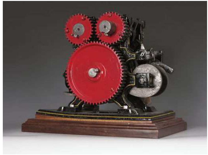
Figure 8.10. 1857 patent model showing the drive gears with their 2:1 ratio. The flywheel and hand crank, seen in the patent drawings, once attached to the shaft of the upper right gear, have been lost, probably in the fire that damaged the model (photo by Allison Munsell, Albany Institute of History and art).
