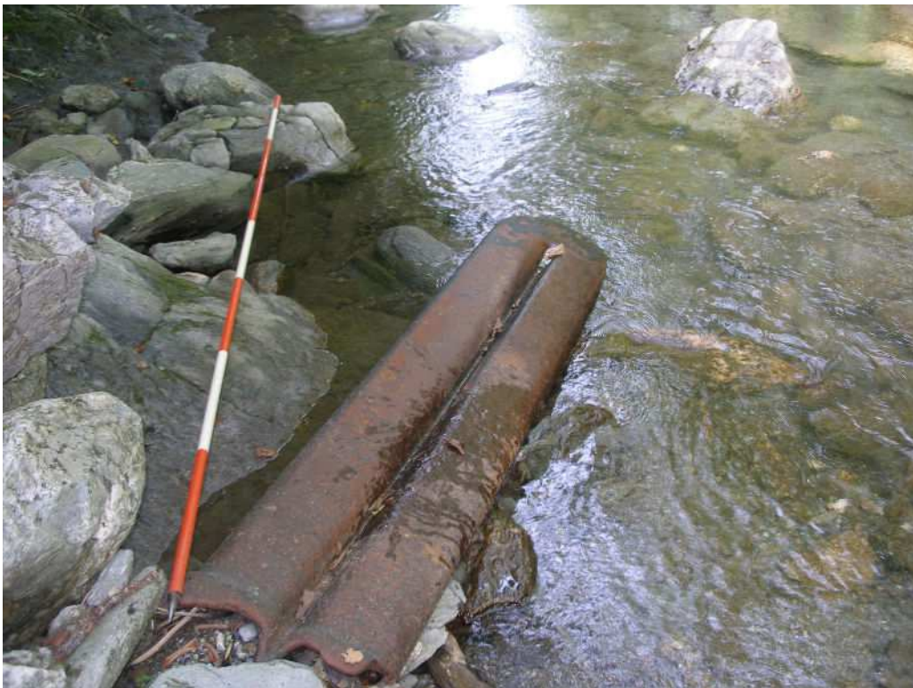
Figure 6.8. A radiator pipe in the nearby Bash Bish Brook. This is one of many examples of important furnace components that may be in danger of washing away over time if they are not documented and monitored before and after seasonal flooding of the brook.
