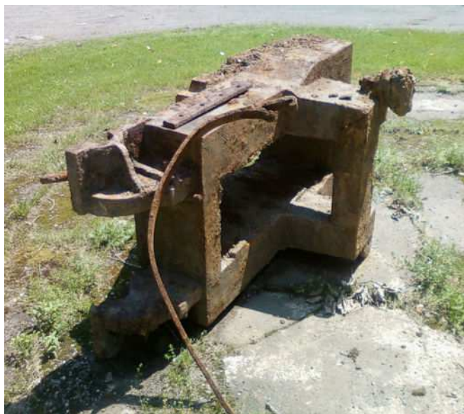
Figure 6.17. An additional piece of the Blake ore crusher discovered during the construction of the Visitors' Center to the south of the ore pond in 2011. This artifact is now next to the boiler fragment near the pattern shop.
