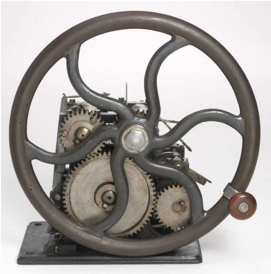
Figure 8.25. The Centennial machine from the drive wheel side showing the 1:2 ratio of the gears. The gear at lower right powered the bending tongue and feed mechanism. The hand crank would have been replaced with a large belt-driven flywheel on the full-sized version (photo by John Yost, New York State Museum).
