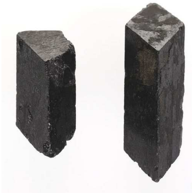
Figure 2.4. Unusual morphology of magnetite crystals (4.7 x 1 x 1.5 cm) resulting from parting along octahedral faces (NYSM 12258).
