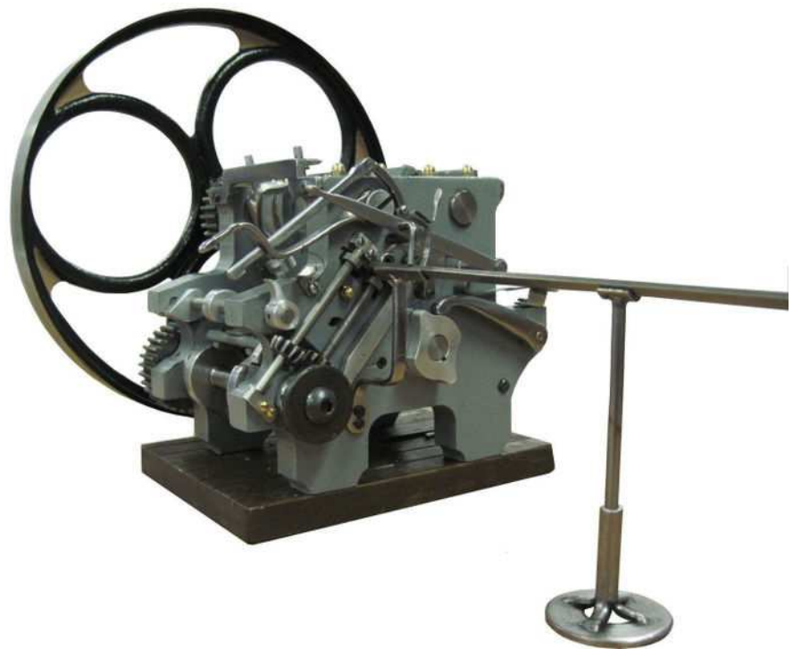
Figure 8.15. Working model of the 1857 rotary horseshoe machine, as seen from the feed side, with a bar of stock lying in the feeding trough waiting to be drawn into the machine by the feed rolls. Photo by John Yost, New York State Museum.
