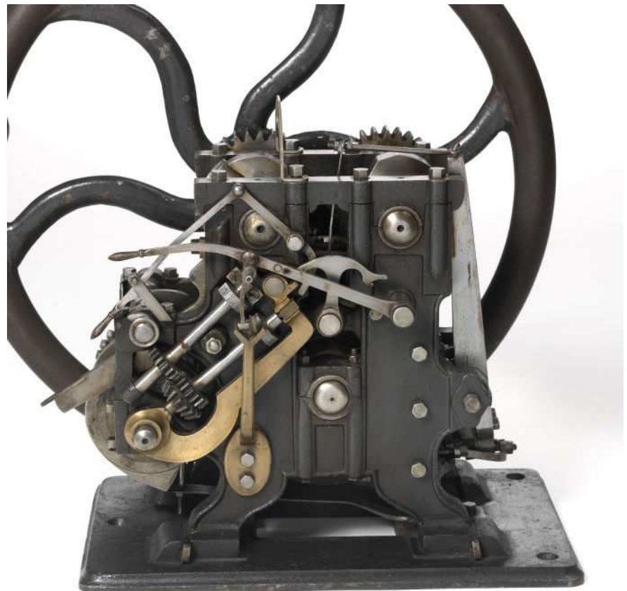
Figure 8.24. The Centennial machine from the feed side. The large beveled gear on the brass movable frame that once drove the feed mechanism is missing. The "indicator" is fitted with a small wheel at the bottom (photo by John Yost, New York State Museum).
