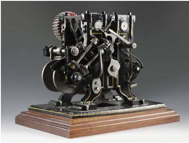
Figure 8.9. Henry Burden's 1857 patent model of the new rotary horseshoe machine, seen from the feed side. The model exhibits some minor damage perhaps from the 1877 Patent Office fire or storage barn fire in 1943. The model has been carefully cleaned and repainted (photo by Allison Munsell, Albany Institute of History and art).
