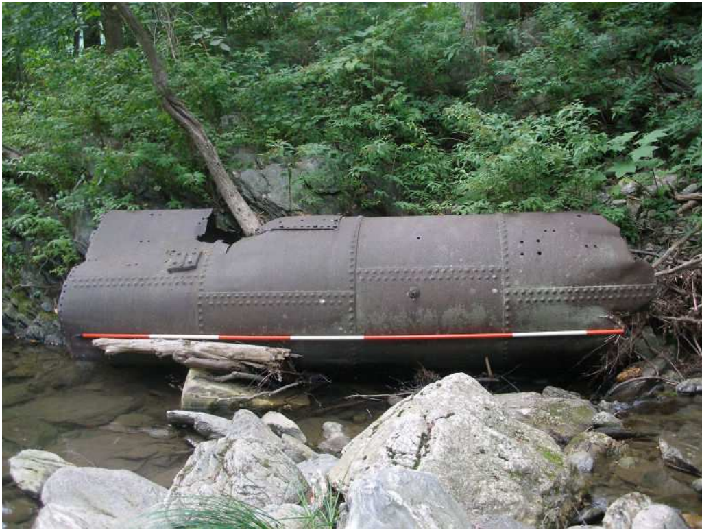
Figure 6.9. A riveted boiler section which was vulnerable to the effects of the brook's eroding shoreline. In 2013 this section of boiler was removed from the stream bank and placed near the pattern shop
