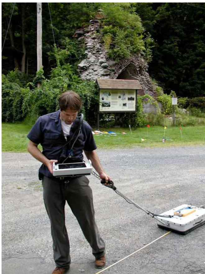
Figure 6.15. Professor John Steinberg pulling his GPR device over the area between the pattern shop and furnace area.
