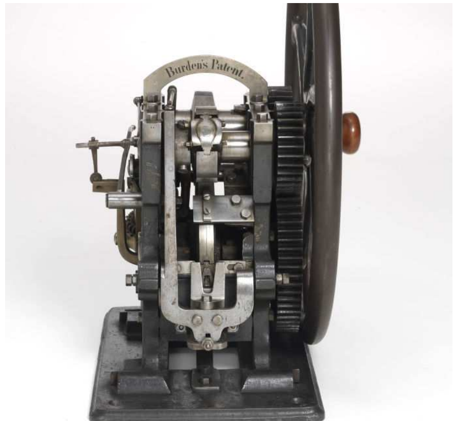
Figure 8.26. The Centennial machine from the rear, showing the large wheel that carried the lower dies (not visible). The line machined on the large wheel was to aid in adjusting the swaging dies to the center of the wheel. The "V" shaped scraper that pulled the shoes free to drop into the flattener is visible below the large wheel, but the flattener itself is hidden behind the "U" shaped yoke at the bottom (photo by John Yost, New York State Museum).
