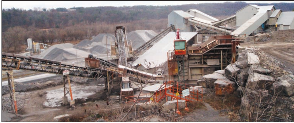
Figure 17. Typical crushing and screening operation. Primary crusher (right) feeds material to secondary crushers and sizing screens. Material is stockpiled by size (background).
