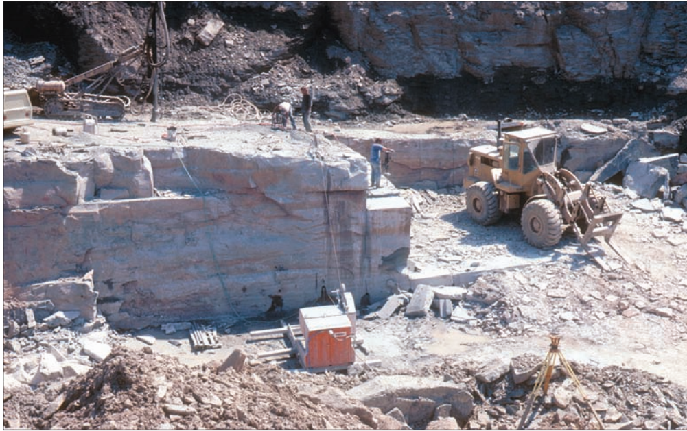
Figure 3. A wire saw is used to quarry blocks of sandstone, commercially known as “bluestone,” for use as dimension stone, Walton, New York. The blocks will be re-sawn to desired size and thickness.
