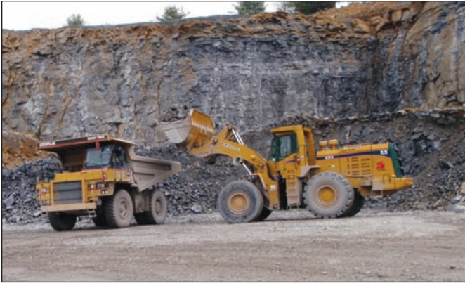
Figure 15. Wheeled loading and hauling equipment is used to move blasted rock to the crushing plant. Courtesy Callanan Industries, Inc.
