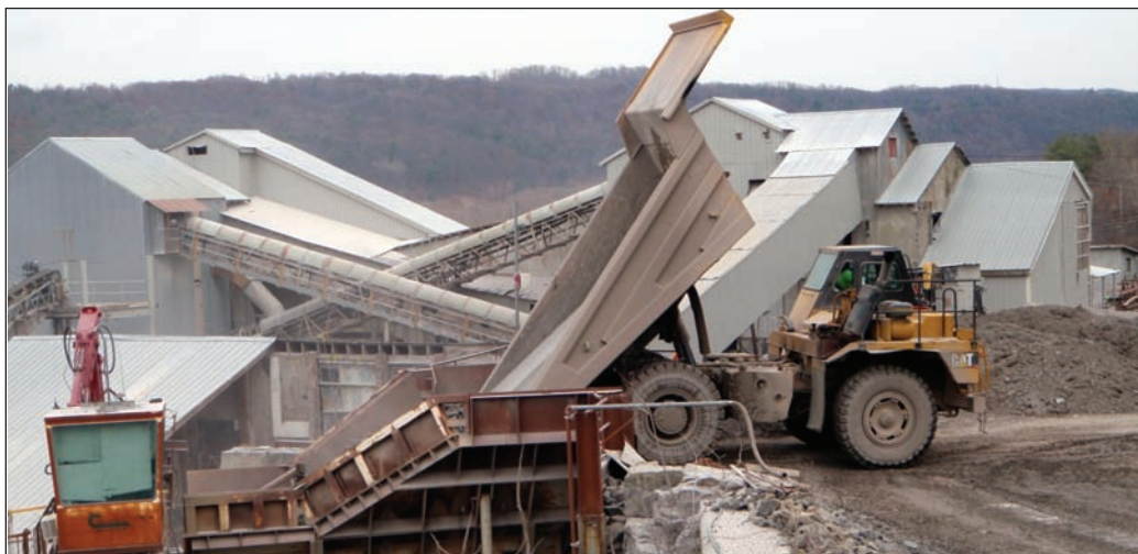
Figure 16b. Rock dumped into primary crusher. Courtesy Callanan Industries, Inc.
