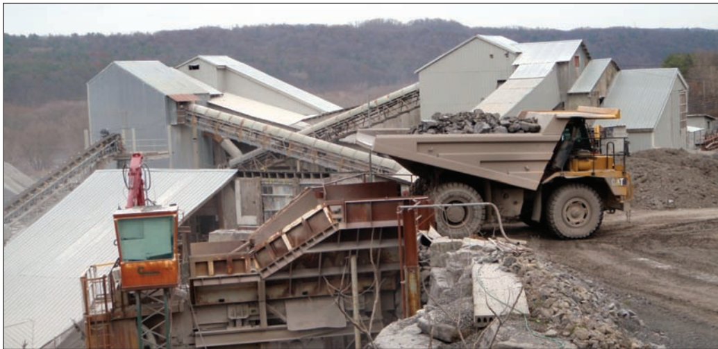
Figure 16a. Truckload of blasted rock at primary crusher. Courtesy Callanan Industries, Inc.
