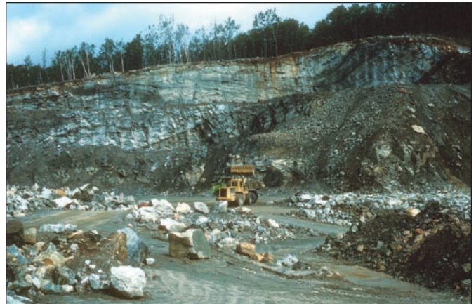
Figure 5. Crushed stone quarry, near Saranac Lake, New York. Rocks being extracted are marble (white) and granitic gneiss (dark).
